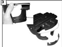
Remove Safety bar from mounting bracket by loosing screws, sliding bar to side, and lifting it off the 2 screws.
